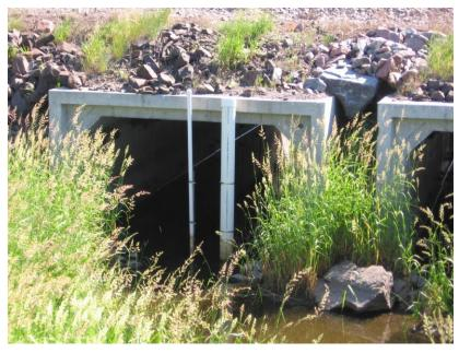
Figure 2. Stilling Wells for Continuous Monitoring Equipment at B75 (Brandt Channel at Hwy 75)
